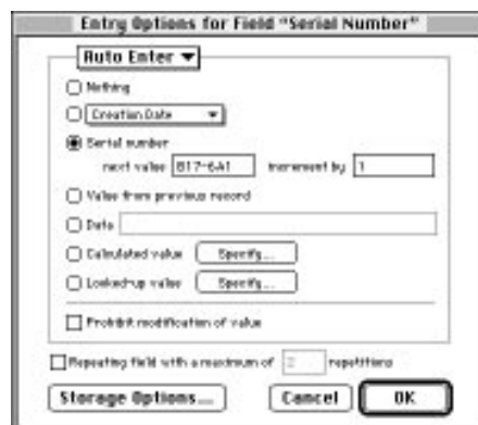
Creating a serial number that contains numbers and letters is easier than you'd think.
